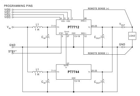
External Capacitors: The PT7744 requires a minimum ouput capacitance of 330µF for proper operation. The PT7744 also requires an input capacitance of 1500µF, which must be rated for a minimum of 1.4Arms of ripple current. For transient or dynamic load applications additional capacitance may be required. For further information refer to the application note regarding capacitor selection for this product.
